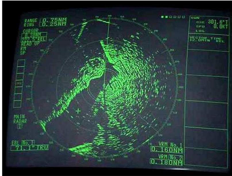
Fig. 3.4 Radar scope image taken from a ship, located at the center of the scope, in a harbor (dark patch through the center) surrounded by land (bright returns). Radar reflections are received only from objects exposed to the central radar dish. Parts of the image occluded by nearer objects show no radar reflections. The thin vertical shadow extending downward from the center is probably due to some obstacle, like the ship's own smoke stack, blocking the radar signal in that direction.
